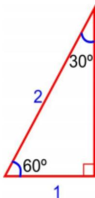
$$\begin{aligned} c^2 &= a^2 + b^2 \\ a^2 &= c^2 - b^2 \\ a^2 &= (2)^2 - (1)^2 \\ a^2 &= 4 - 1 = 3 \\ a &= \sqrt{3} \end{aligned}$$
