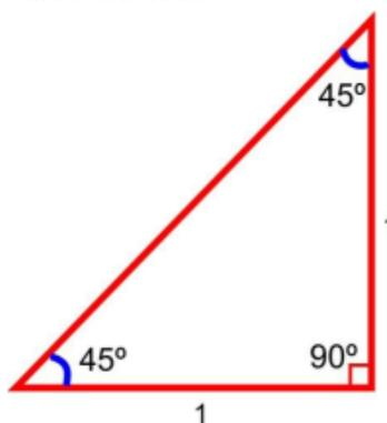
$$\begin{aligned} c^2 &= a^2 + b^2 \\ c^2 &= (1)^2 + (1)^2 \\ c^2 &= 1 + 1 = 2 \\ c &= \sqrt{2} \end{aligned}$$
